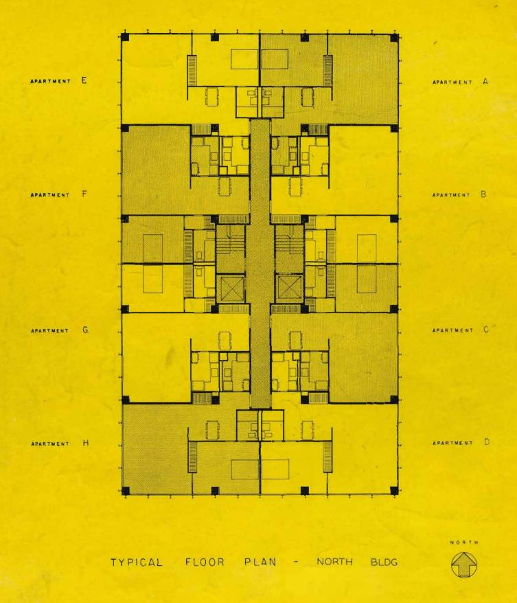
These typical floor plans show the  $3\frac{1}{2}$  room apartments in the North Building and the 6-room apartments in the South Building. Note the symmetrical design of both buildings which not only permits economy in construction but also makes full use of the abundant light and breeze and the exhibitance view inherent in the location.
